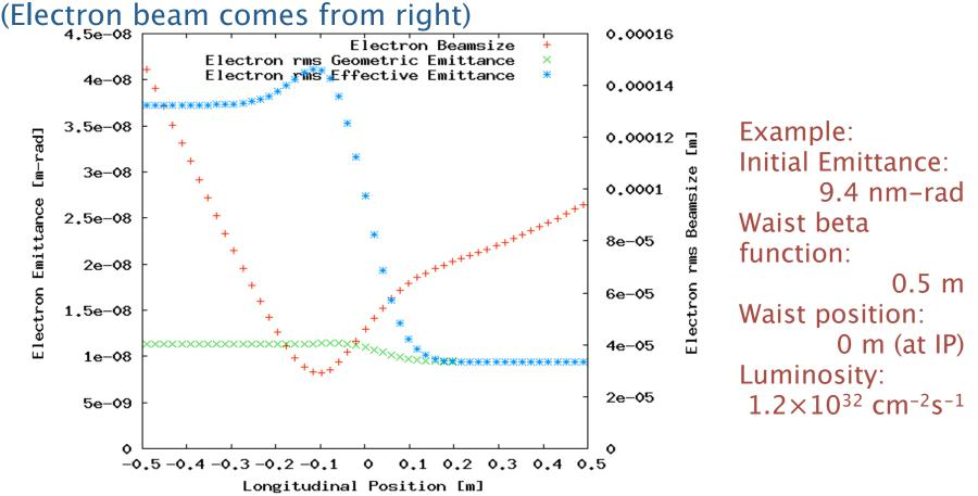
Effective emittance growth during collision due to mismatch between the electron distribution and design lattice. This is main effect comparing with the geometric emittance growth due to pure nonlinear effect.
