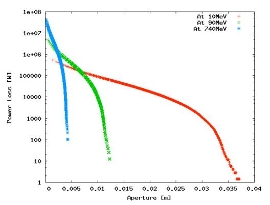
The required aperture if 1KW power loss is required.
