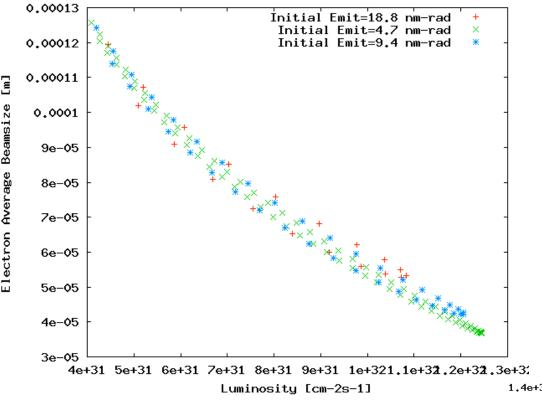
In order not to drive the proton beam unstable, the electron beam size must be controlled.
